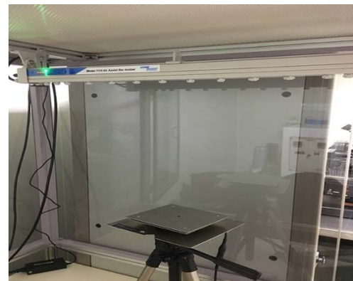
Figure 3: Air assist bar ionizer installation with CPM plate Ionizer needed small adjustment from the factory set due to humidity and temperature differences in
